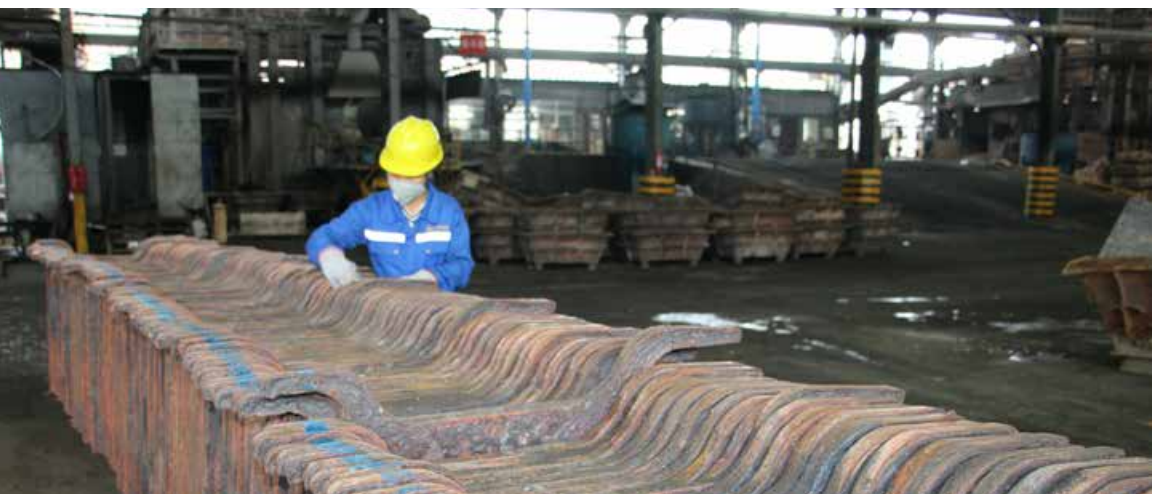
EXAMINING THE QUALITIES OF ANODE PLATES AT JIANGXI ZILI ENVIRONMENTAL PROTECTION TECHNOLOGY CO. LTD. PHOTO BY LE LAN
