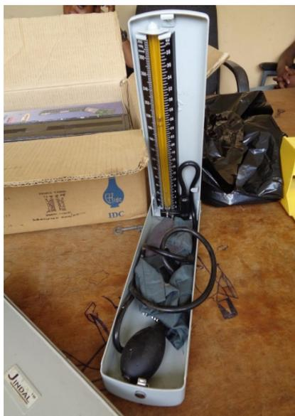
(A mercury containing blood pressure meter or sphygmomanometer)
